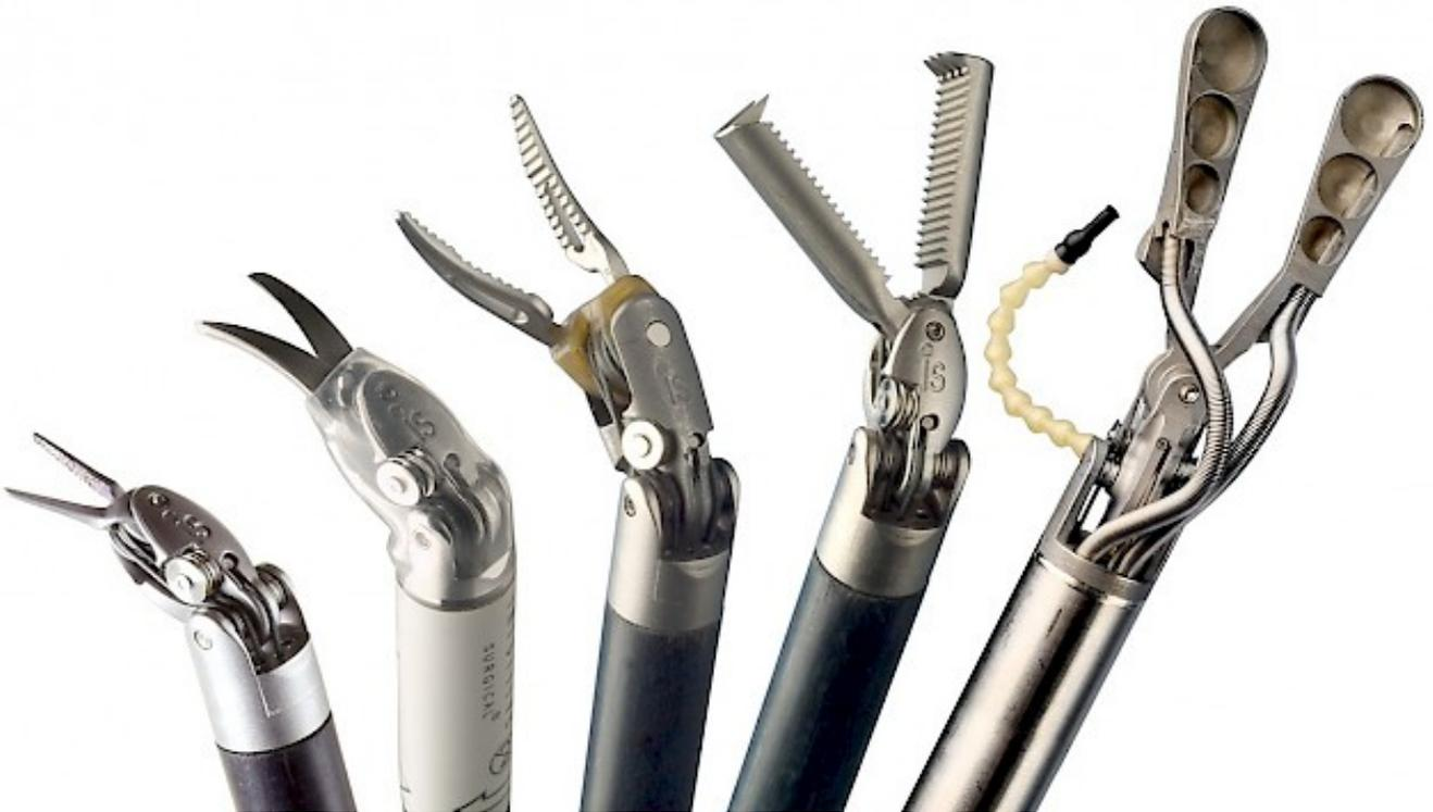
Attachments such as scalpels, scissors, Bovie cauterizers, and fiberoptic cameras aid the da Vinci robotic system in performing surgery.
